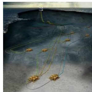
Field layout of the Goliat subsea field in the Barents Sea. Illustration: Eni Norge AS
