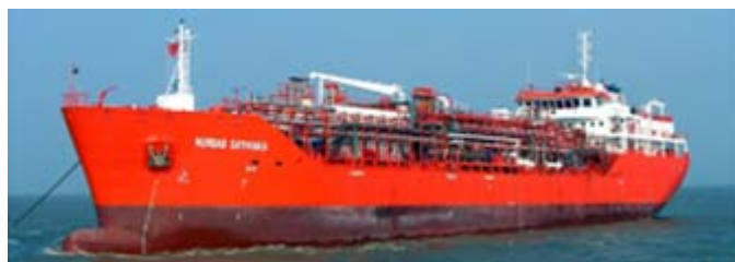
Norgas Cathinka – 2nd Wintergas vessel delivered in the end of October 2009. The ship is a Special. LPG/Eth/Chemical combo carrier – 5 800/ 9 600cbm.
